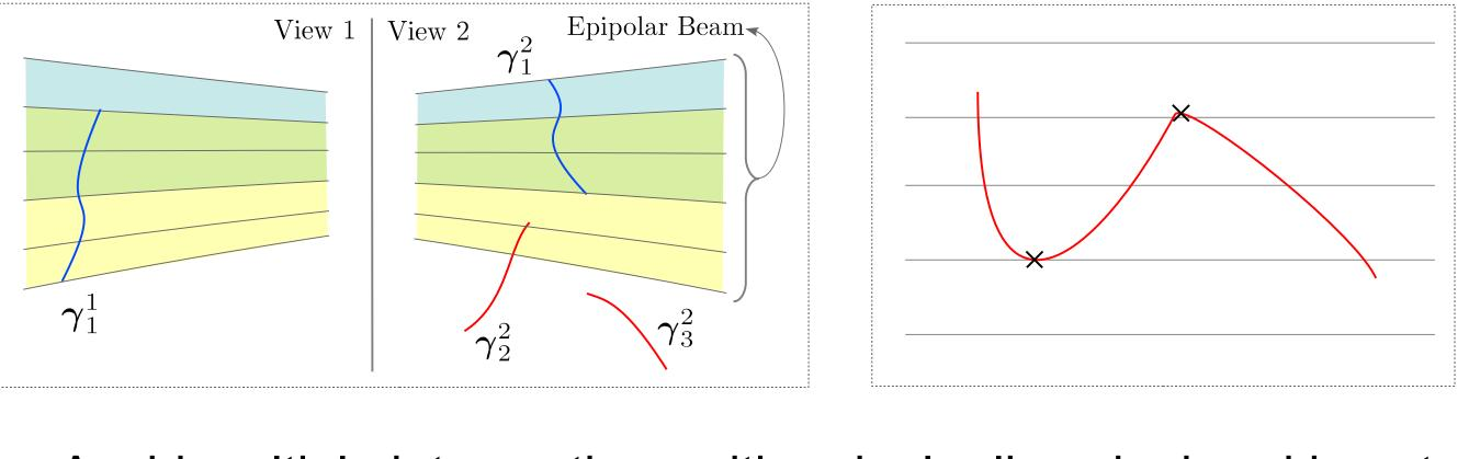
• Avoid multiple intersections with epipolar lines by breaking at epipolar tangencies
